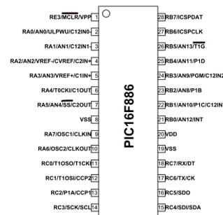
Fig -2: PIC 16F886 Microcontroller
